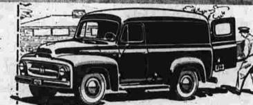
specialists in the multi-stop field. Hi-tensile steel body has 215 cubic feet capacity. Drop frame construction allows low stepwell, 78-inch headroom in through aisle. Four models with 7-foot bodies on 115-inch wheelbase, GVW ratings, 5,400 to 9,000 lbs. New METRO-Matic
